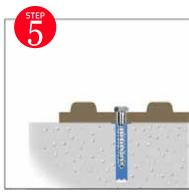
Align the tread in the desired position. If you are installing a nosing, make sure that it fits snugly at the edge of the stair. If you are installing a tread, set it back roughly ½" from the edge.
